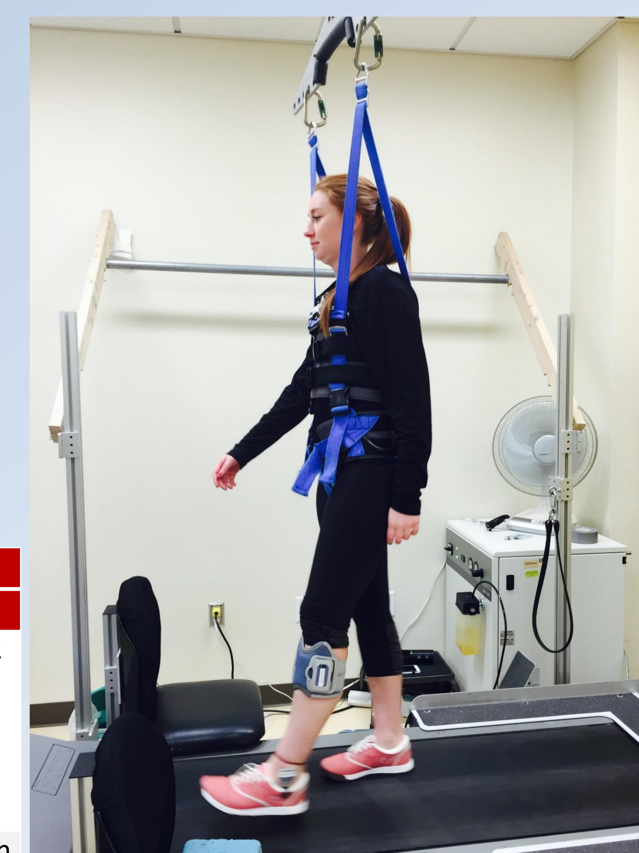
Figure 2: Lateral view of Therastride Body Weight Supportive Treadmill System with use of left Bioness L300 stimulation cuff.
