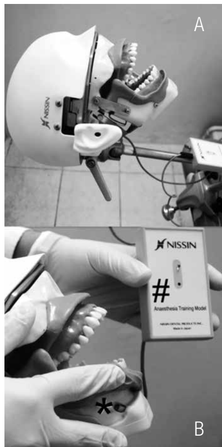
Figure 1. The conduction anesthesia simulation model (CAM) is a typodont with anatomical landmarks including the mandibular ramus. The simulation model is fixed to a phantom head which is then is mounted on the backrest of the dental chair (A). It includes an electronic device (B,#) that produces a signal when the dental needle touches the metallic electronic sensor (B,*).
