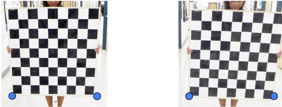
Figure 10. Points outlining the horizontal bottom of the large calibration board from stereo-pair images (0.914m x 0.914m board with 9 x 9 squares (squares 0.098 x 0.098m)) in the A position. Points were triangulated using the Matlab stereo-calibration program, and the Euclidian distance in pixels (known length 0.914m) was used to scale seal photographs.
