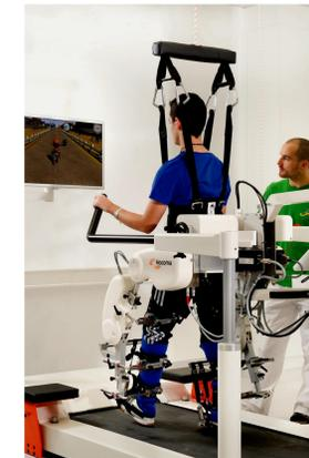
Figure 1: Depicts patient on a robot-assisted gait training device. Picture: Hocoma, Switzerland. <http://www.hocoma.com/en/>
