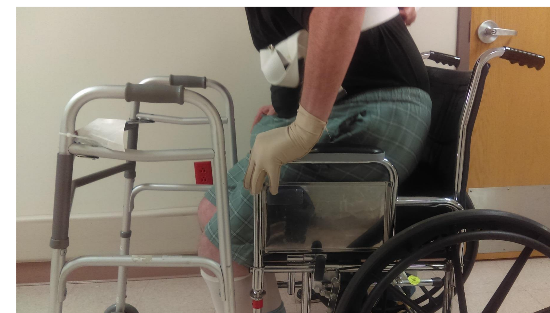
Figure 1: Sit-to-stand transfer with spring-loaded wheelchair seat
